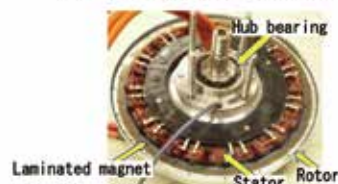
Example of an EV main motor with laminated magnet (in-wheel motor by e-Gle Co., Ltd.)
